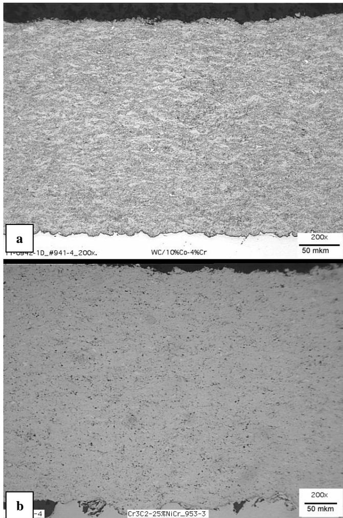
Figure 4: Micrographs of WC-10Co-4Cr (a) and Cr<sub>3</sub>C<sub>2</sub>-25NiCr coatings (x200, etched)
