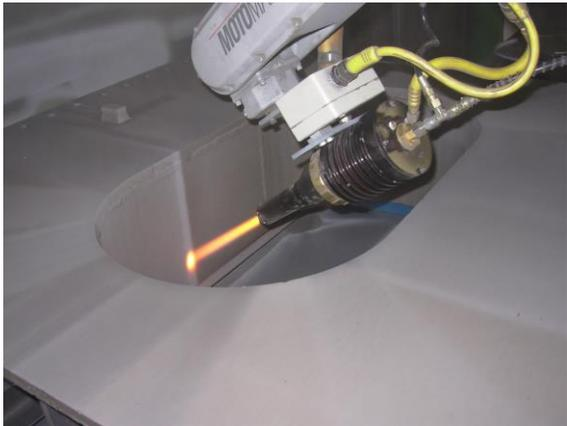
Figure 5: Application of the WC-10Co-4Cr coating with the AK-07 HVOF gun onto restriction grid with orifice (upper slide plate of the catalyst tower)
