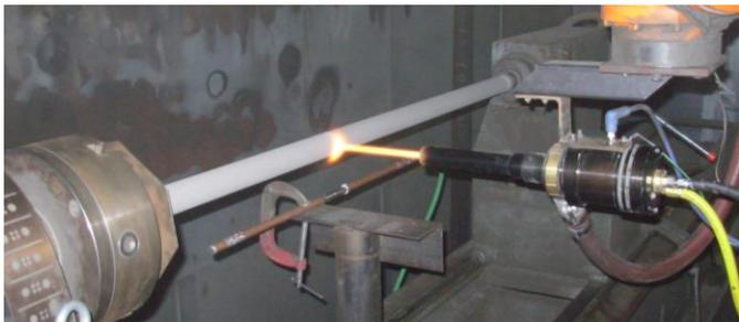
Figure 6: Application of the WC-10Co-4Cr coating with the AK-07 HVOF gun onto hydraulic rod of sea dock crane
