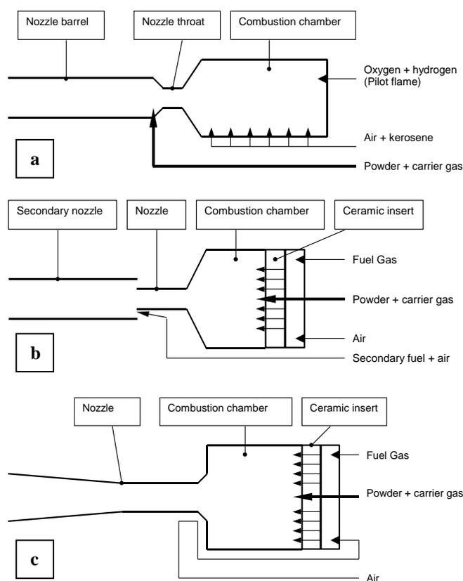
Figure 1: Principal schematics of HVAF guns: AeroSpray (a), SB9300 and M3 (b), AK-07 and AK-06 (c).
