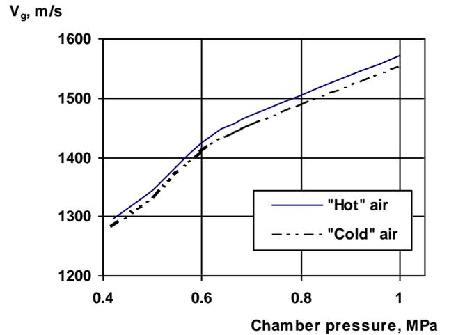
Figure 2: Results of calculations of the influence of absolute combustion chamber pressure on the gas velocity  $V_g$  at the exit of the de Laval nozzle
